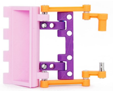
Linkage system driven by servomotors
